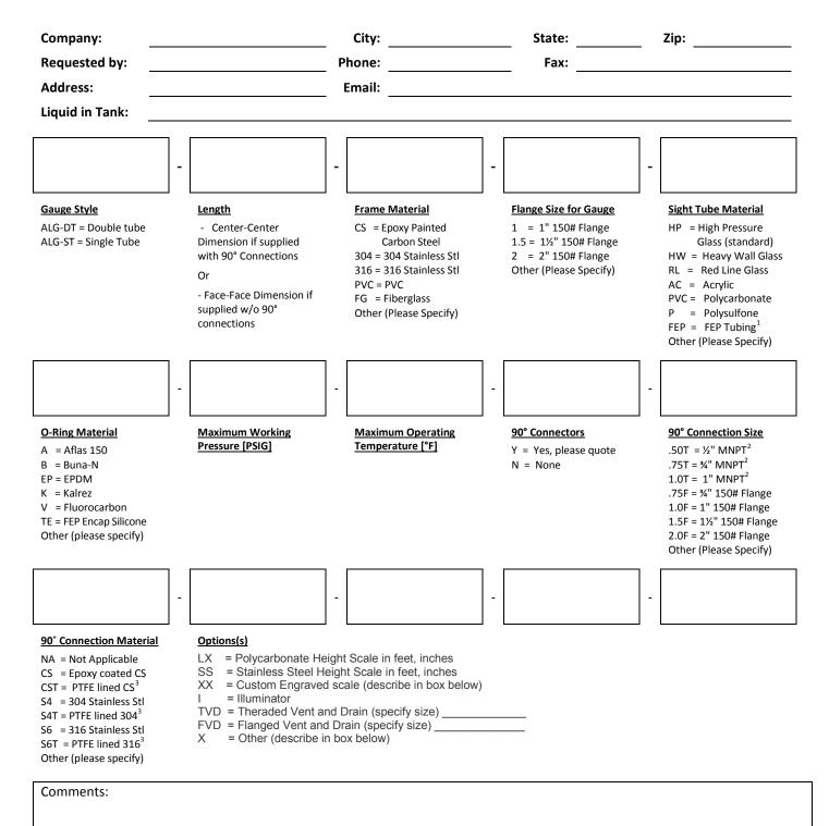
**Example:** ALG-DT-48-316-1.5-RL-TE-175-100-Y-1.5F-S6-LX-1/2"TVD is a double tube gauge, with a center to center dimension of 48", frame material is 316 SS, 1.5" 150 LB. flanged connections, red-line glass, FEP Encapsulated Silicone O-rings, a maximum working pressure of 175 psig at 100°F, with 1.5" 150# flanged 316 SS 90 degree connectors, a polycarbonate height scale in feet/inches, and 1/2" FNPT vent and drain connections.
